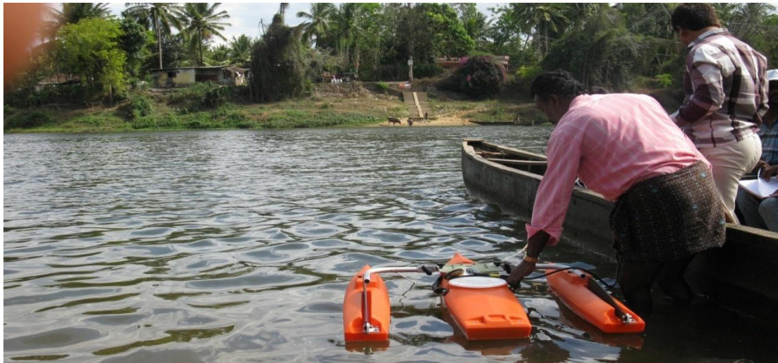
AUTOMATIC DOPPLER CURRENT PROFILER FOR FLOW MEASUREMENT
