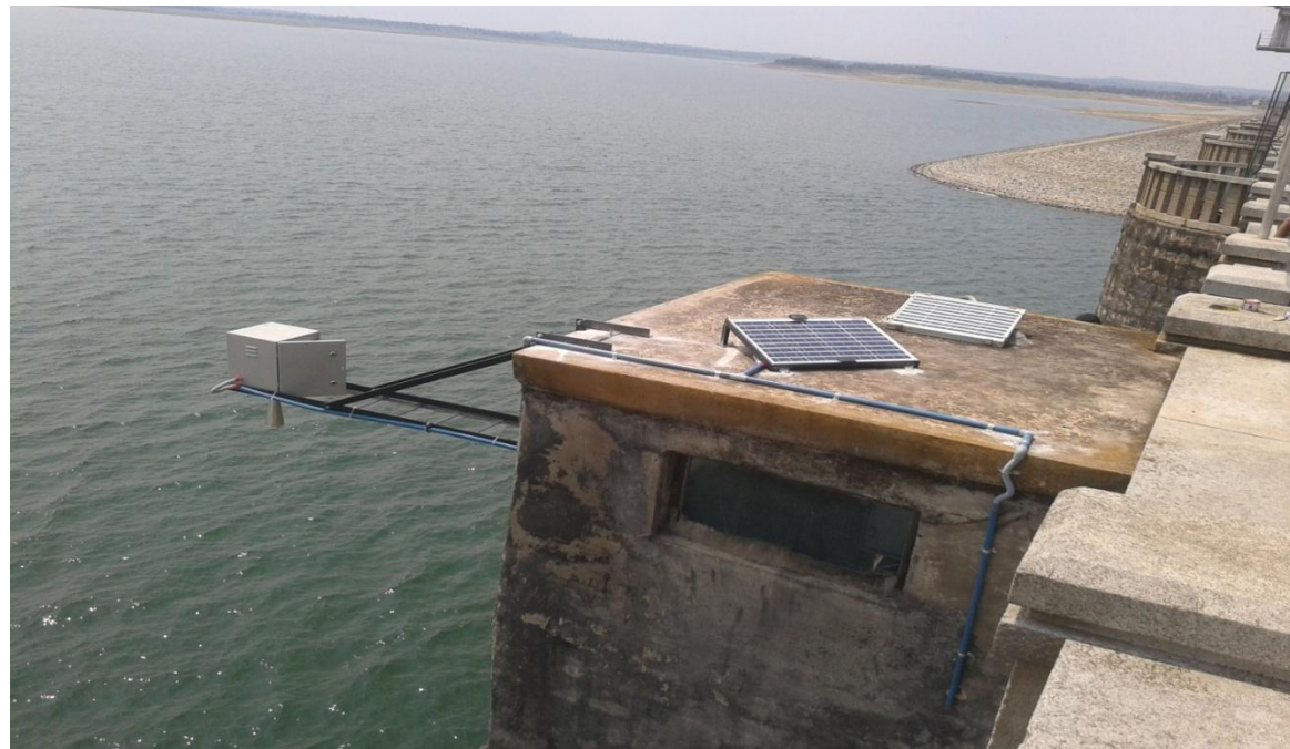
NON CONTACT RADAR SENSOR FOR LEVEL MEASUREMENT
